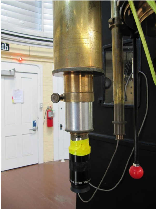
The finder scope eyepiece and one of the red knobs used to move the telescope.
