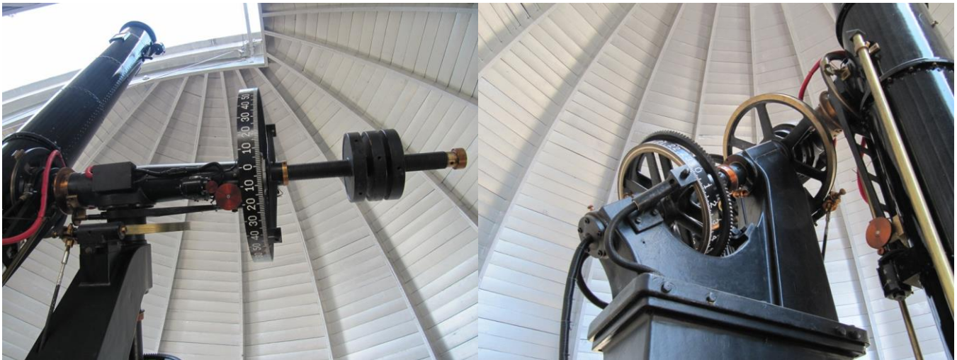
The Declination Axis and Setting Circle
